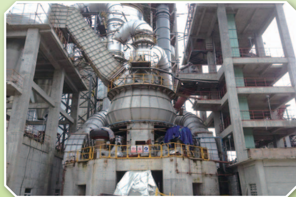
The raw materials vertical mill built by the Group in Papua Barat, Indonesia
